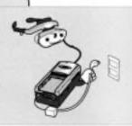
Always use the designated AC power adapter (included with the product). Using other AC power adapter may cause damage or fire.
