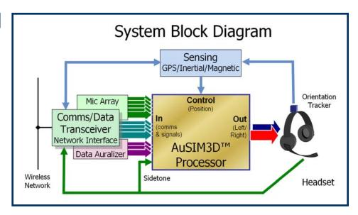
Figure 2 - Common features of all 3DVX configurations
